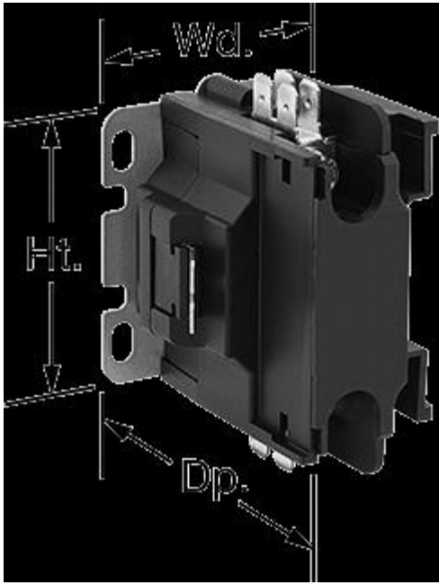
Infrequent-Cycle High-Current Relay SPST-NO, 120V AC Input, 25A Full Load @ 600V AC
